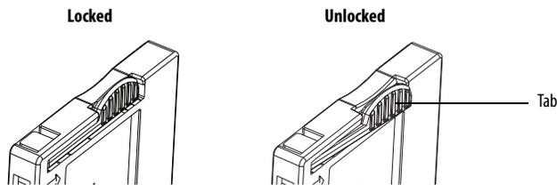
2. Align the end cap with interlocking pieces on the last installed terminal base.
