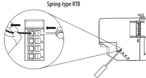
**IMPORTANT** When you insert a screwdriver to disconnect wires, follow the entry angle on the right-side terminal of a spring-type RTB.
