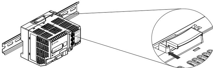
3. Position the adapter so that the back of it faces the DIN rail.
