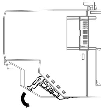
5. Press down the DIN rail latch.
