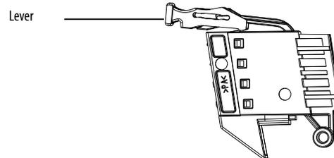
2. Insert the Power RTB into the RTB slot as shown in the graphic and press it until it clicks.
